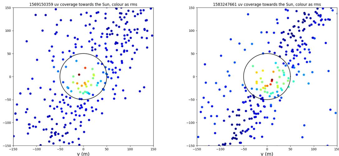
Figure 8: uv-coverage towards the Sun, showing the rms per baseline
