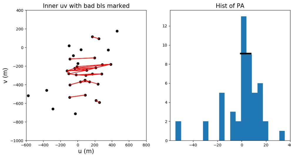
Figure 7: Inner core with affected baselines and histogram of their position angles
