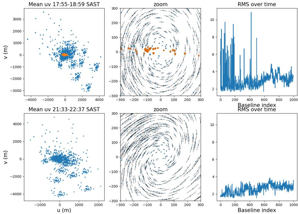
Figure 6: uv-tracks showing the affected baselines lining up towards the Sun for dataset 2
