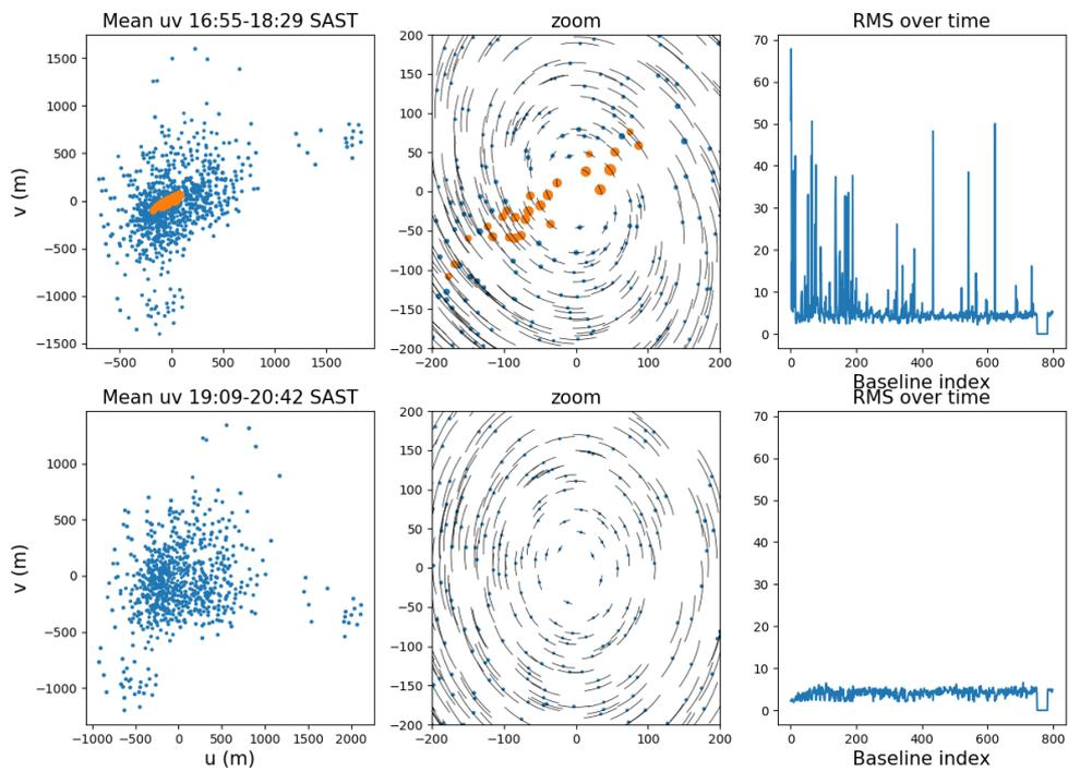
Figure 5: uv-tracks showing the affected baselines lining up towards the Sun for dataset 1
